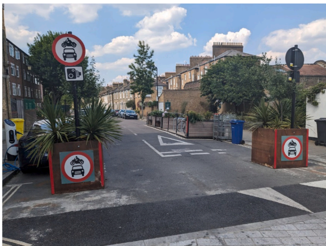
Fig. 1. Automatic Number Plate Recognition (ANPR) enforced modal filter in a LTN.
