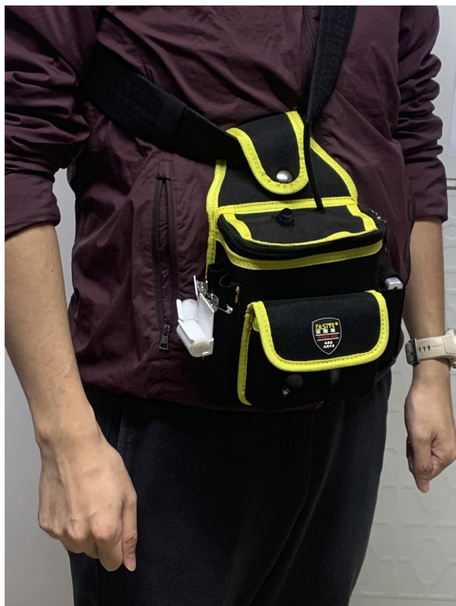
Fig. 3. Illustration of personal monitoring kit worn by a researcher. All battery-operated personal monitors and a GPS tracker were contained in the small messenger bag, and measured personal pollution levels through conductive tubing.
