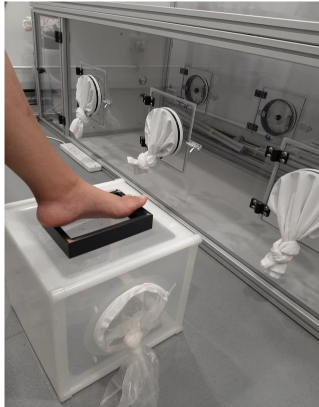
Figure 1: Foot on cage assay, the participant's foot is placed on top of a cage containing 20 female mosquitoes, the plastic grid prevents the participant from being bitten.
