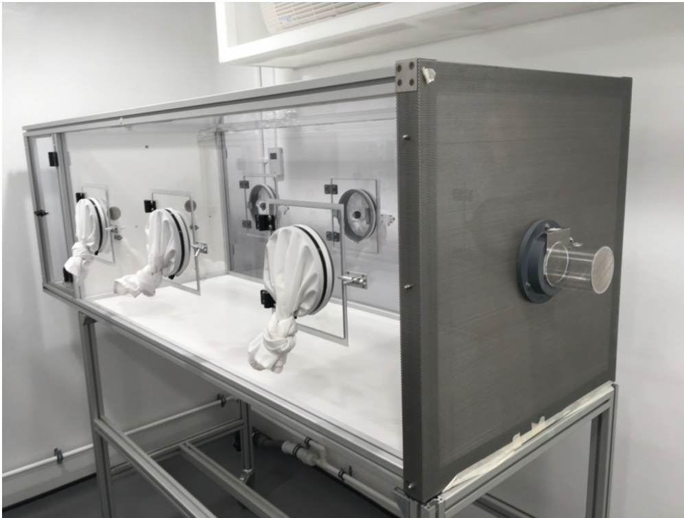
Figure 10. Overview of the dual choice wind tunnel used for behavioural experiments to test attractiveness to Anopheles coluzzii mosquitoes using worn socks in the UK cohort. On the right-hand side is the release chamber. Traps to catch the mosquitoes are behind the white panel on the left-hand side.
