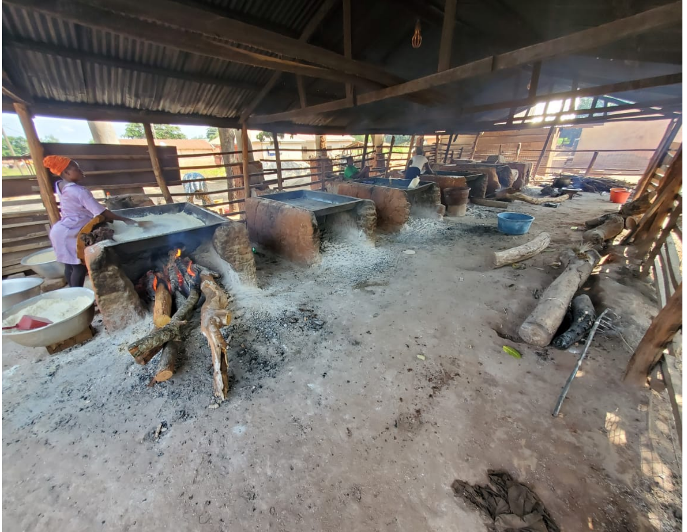
A gari worker using a small foam cushion to lean on the side of a hot biomass stove to process the gari.
