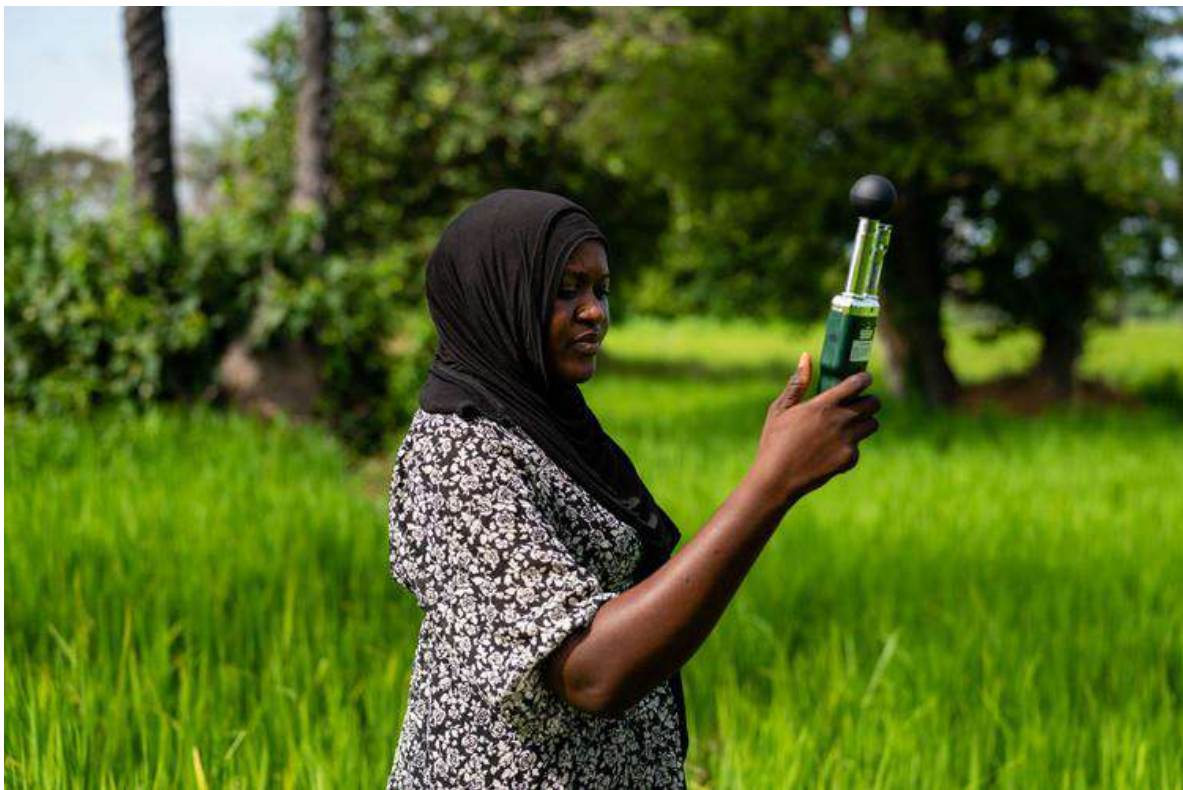
Figure 1: Tida Samateh using the Extech 200 heat stress meter to measure heat stress in a rice field.
