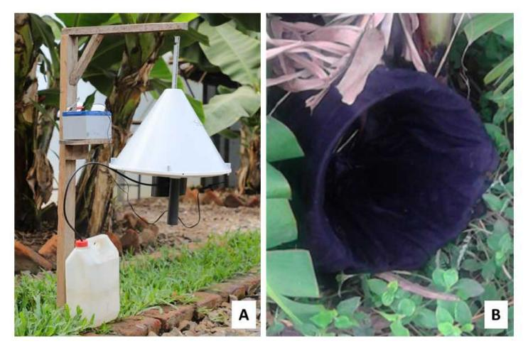
Fig 2. Mosquito Traps: Odour-baited Suna® trap, for sampling host-seeking mosquitoes (A) and Resting bucket trap (RBu) for resting mosquitoes (B). https://doi.org/10.1371/journal.pone.0245750.g002
