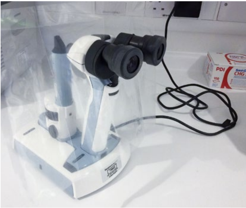
Figure 3 Portable slit lamp breath shield. UK
