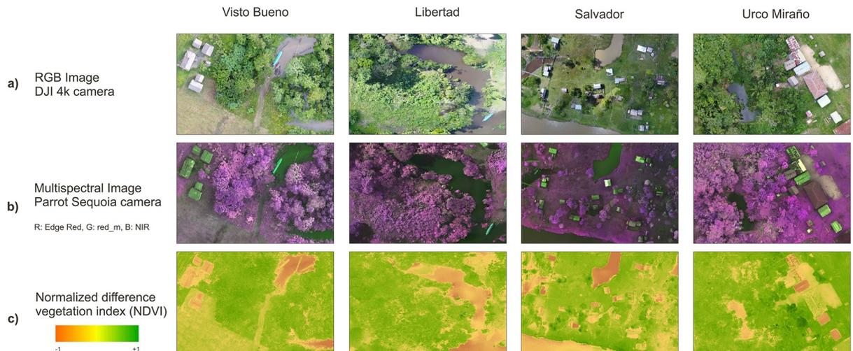
**Fig 4. Orthomosaic scenes of the communities of Visto Bueno, Libertad, Salvador, and Urco Miraño using a) RGB imagery, b) Multispectral imagery, and c) Normalized Difference Vegetation Index (NDVI).** Orthomosaics based on drone imagery were constructed in AgiSoft Photoscan Pro (<https://www.agisoft.com>) and mapped in QGIS.
