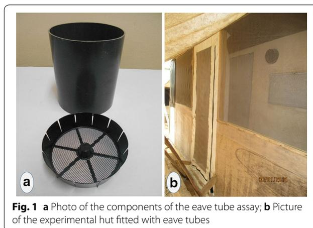
**Fig. 1** a Photo of the components of the eave tube assay; b Picture of the experimental hut fitted with eave tubes
