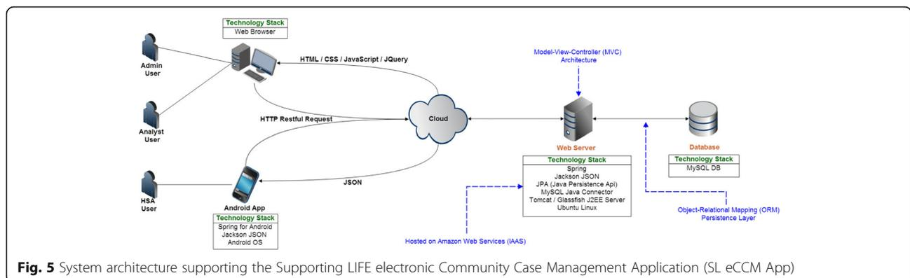
**Fig. 5** System architecture supporting the Supporting LIFE electronic Community Case Management Application (SL eCCM App)
