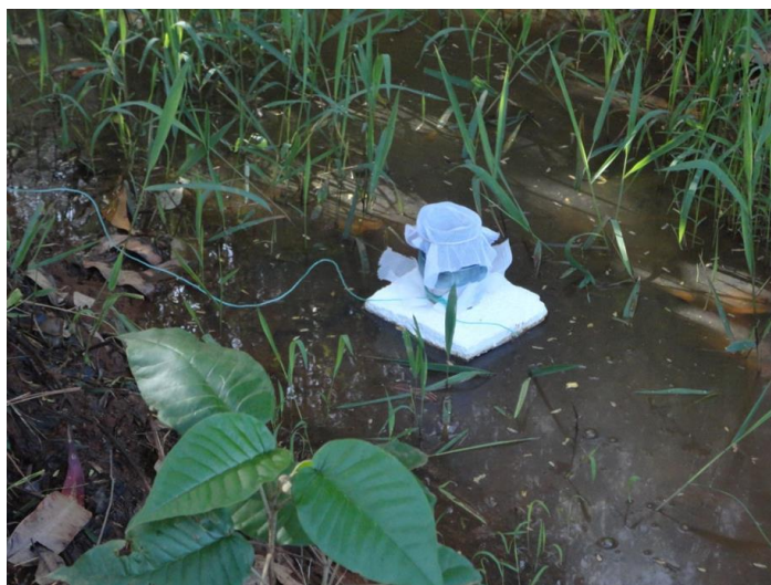
Figure 4.7: Floating cup for exposure of insectary-reared larvae directly in aquatic habitats
