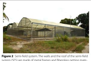
system (SFS) are made of metal frames and fiberglass netting material. The SFS has two sections separated by heavy-duty polyurethane. Each of these sections contains one experimental unit.
