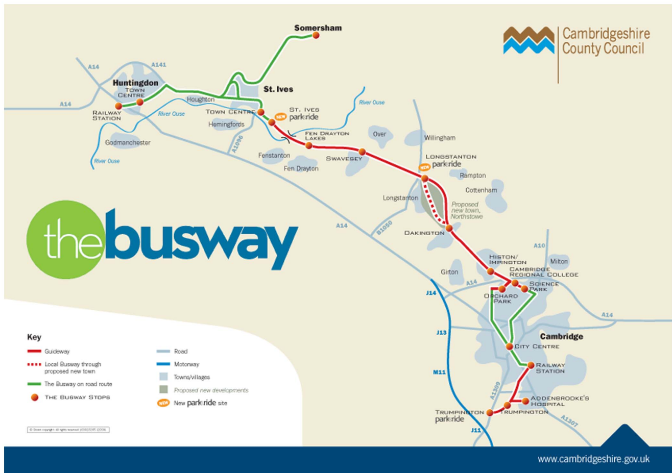
Figure 1. The Cambridgeshire Guided Busway. Reproduced with permission from Cambridgeshire County Council and Stagecoach. The guideway runs from St Ives to the northern edge of Cambridge city, and from Cambridge railway station south to Addenbrooke's Hospital and Trumpington. Through the city centre, and north of St Ives, guided buses join the road network. doi:10.1371/journal.pone.0069254.g001
