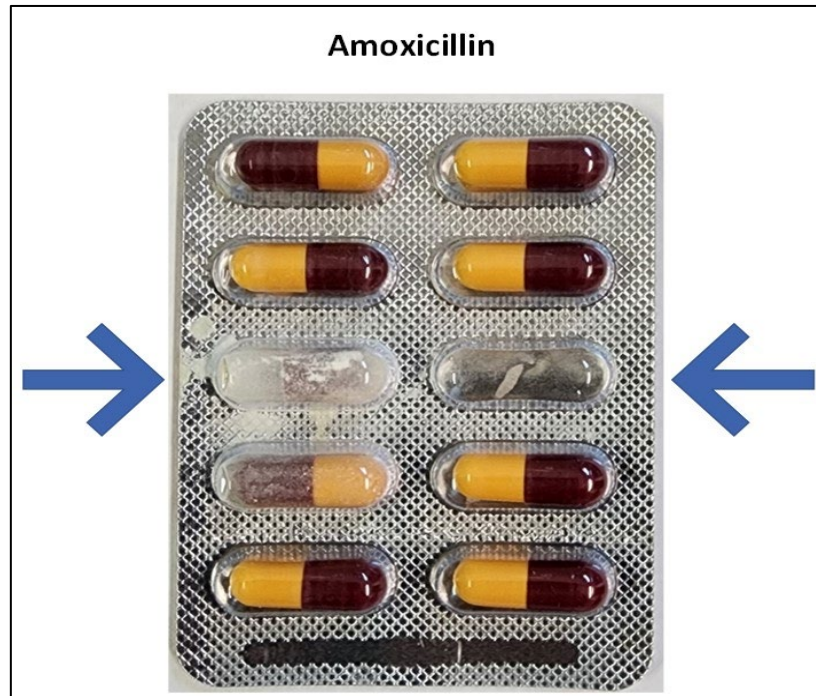
Figure 3: Image depicting a defective amoxicillin sample. Blue arrows indicate the absence of capsules in the blister.
