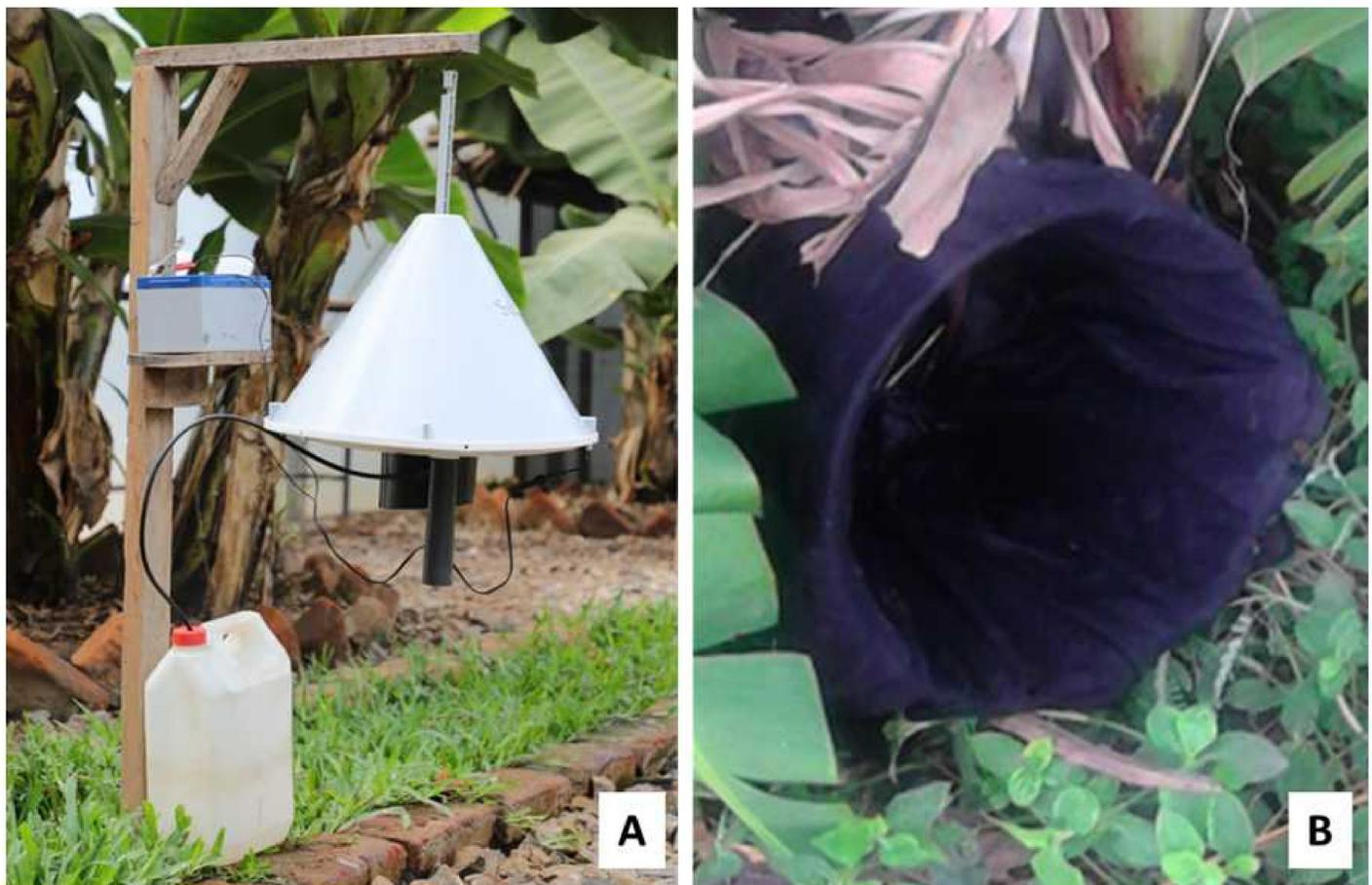
**Fig 2. Mosquito Traps: Odour-baited Suna® trap, for sampling host-seeking mosquitoes (A) and Resting bucket trap (RBU) for resting mosquitoes (B).**
