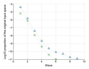
**Fig. 4.** Proportion of the samples drawn at random in the original simulator input space, that are non-implausible after *k* waves of history matching (the emulated variance methodology proposed achieved the same reduction of non-implausible space in three fewer waves):  $\Box$ , emulated variance;  $\Delta$ , fixed variance
