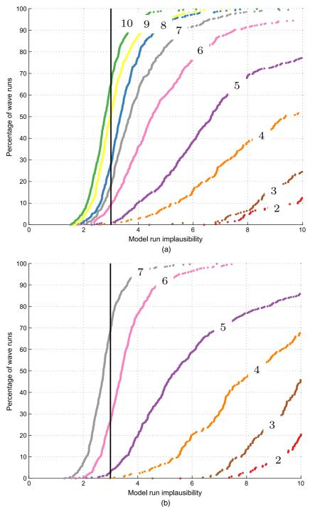
**Fig. 3.** Cumulative distribution function of simulator run implausibility  $I_{\mathcal{R}}(\mathbf{x})$ , by wave (each curve represents the percentage of each wave's simulator runs with an  $I_{\mathcal{R}}(\mathbf{x})$  less than the value indicated by the horizontal axis; the numbers on the curves indicate the wave number): (a) fixed variance; (b) emulated variance
