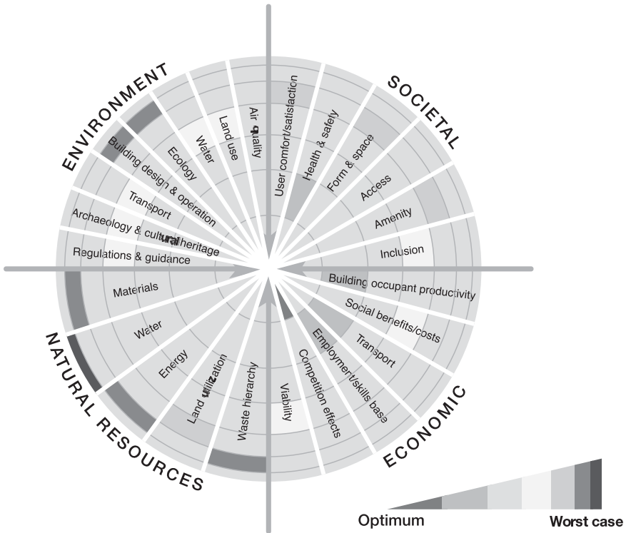
Fig. 12.5 The Sustainable Project Appraisal Routine (SPeAR) developed by Arup
