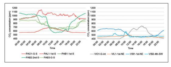
Figure 3. Diurnal CO<sub>2</sub> concentration profiles in PA (left) and VI (right).
