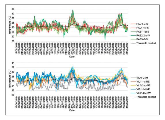
Figure 5. Temperatures (hourly resolution) in monitored PA (top) and VI (bottom) locations, with threshold comfort temperature shown.
