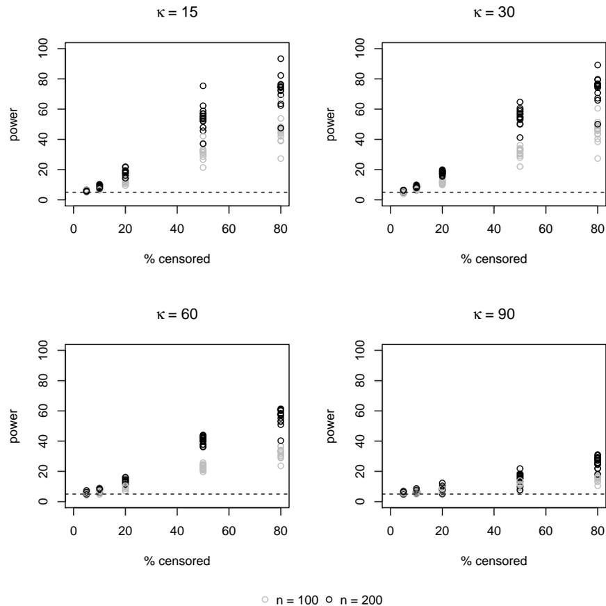
**FIGURE 3** Test for identification of event-dependent observation periods: proportion censored plotted against power. The four panels show results for different lengths of  $\kappa$ . Only results with censoring days uniformly distributed between the event day and 300 are shown.
